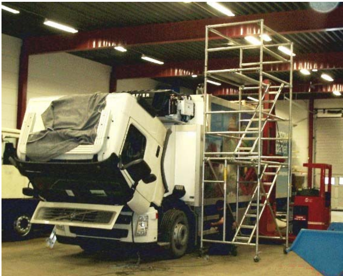
Kylindustri garage. Rolling scaffolds are used for repair and recharge both aggregates of refrigerated vehicles and MAC systems on the roof of buses.
