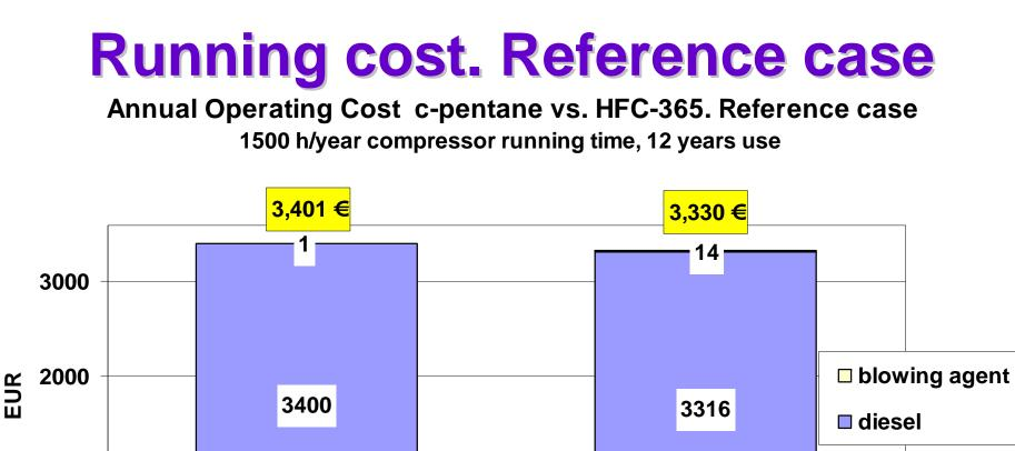
Caused by lower diesel consumption, (partial) annual running cost of vehicles with HFC-blown foam is lower. This difference is not compensated by higher (annualised) cost of blowing agent.
