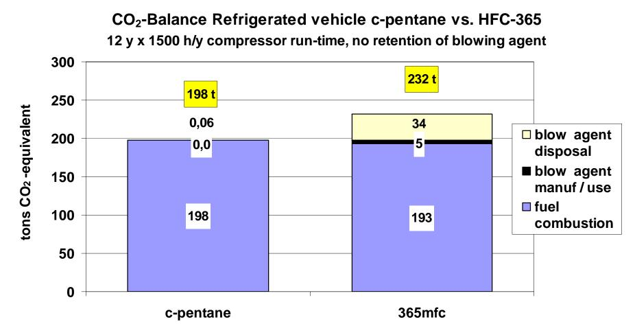
Due to (by 2.5%) higher insulation and hence less diesel combustion, lifetime  $CO_2$  output is lower in HFC case. This advantage is over-compensated by direct blowing agent emission with high GWP. Note: No retention of blowing agents at end-of-live is assumed (today's reality). Lifetime: 12 years.
