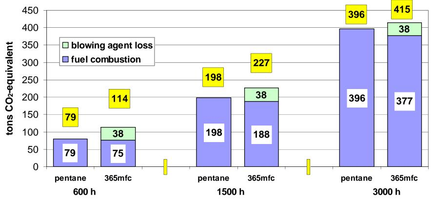
Higher GHG emissions with HFC even at extremely long run-times (3000 h compressor "on" ~ 9000 h cooling)
